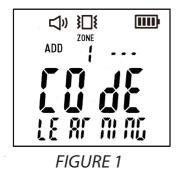
**NOTE:** Each sensor can only occupy one zone of the PR-4000. If you program a sensor more than once, it will remember the last zone it was programmed to and will no longer be programmed to the previous zone.
