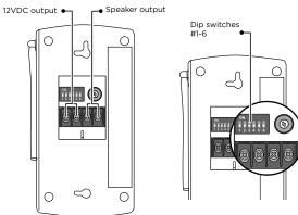
The Di2000R-A is provided with an internal speaker and auxiliary speaker output terminals marked SPKR. The volume knob controls both the internal and auxiliary speakers.
