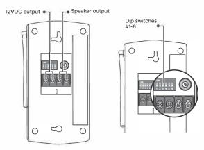
A set of additional 12VDC output terminals are provided for additional buzzers, strobe lights, sirens, or other 12VDCdevices. Please observe marked (+/-) polarity when attaching additional devices. The output time may be set for 1-second or 5-seconds by dip switch in position 5 on the receiver only. The OFF (down) position is 1- second and ON (up) position is 5-seconds.
