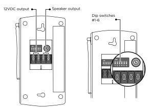
A set of additional 12VDC output terminals are provided for additional buzzers, strobe lights, sirens, or other 12VDCdevices. Please observe marked (+/-) polarity when attaching additional devices. The output time may be set for 1-second or 5-seconds by dip switch in position 5 on the receiver only. The OFF (down) position is 1- second and ON (up) position is 5-seconds.
