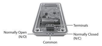
After inserting the wires, tighten the terminals with a small screwdriver.
