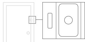
2. Use your fingernail or a flathead screwdriver to pry open the magnetic contact's cover.
