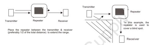
\*\*Do not place repeaters directly in-line with one another as this could cause oscillation.
